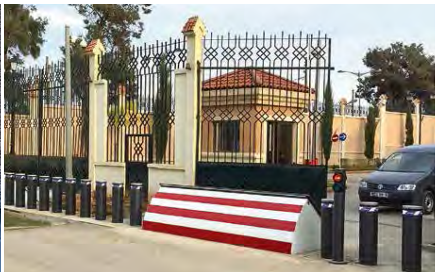
No access: This entrance is protected with fixed bollards and a road blocker.
